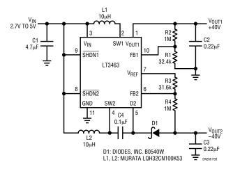
Figure 3. 2.7V to ±40V Dual Output Converter
