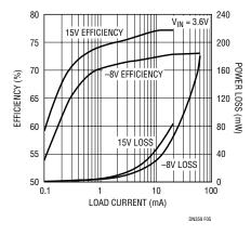
Figure 5. Efficiency and Power Loss for the Circuit in Figure 4
